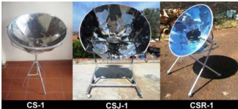
Fig. 2. Solar Cookers CPC of revolution
